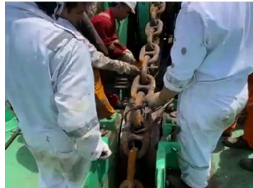
Figure 3. Inserting iron in the anchor chain on the windlass drum
